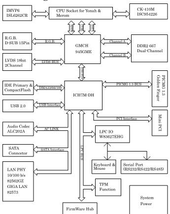
Figure 2.2. Block Diagram
